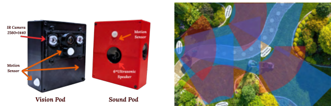
Figure 1: (a) InvisibleFence: Vision Pod and Sound Pod (External deterrent modules); (b) The deployment of pods in a garden and their coverage.
